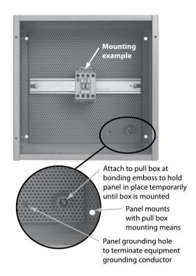
Panel is formed to provide 7/16-in. space off back of pull box for component mounting screw clearance and includes a grounding hole to terminate equipment grounding conductors. Ideal for mounting components that require infrequent access such as control transformers, terminals and contactors.
